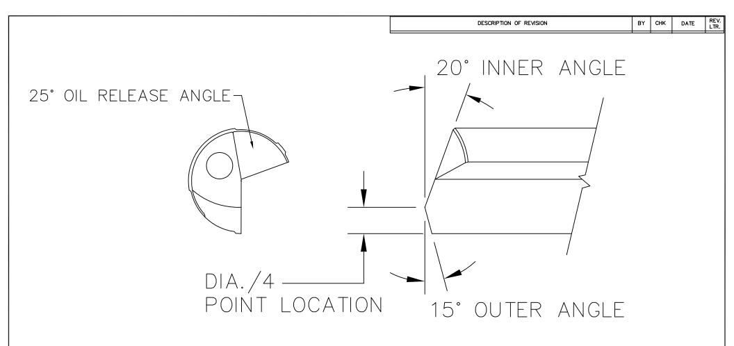
IN ALUMINUM AND BRASS, USE THIS GRIND WITH 'R4' OR 'R2' O.D. CONTOUR
